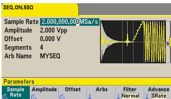
Waveform generator display of the desired sequence.
