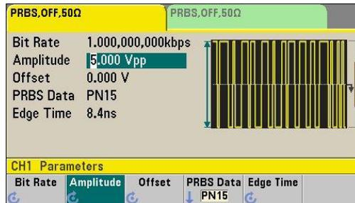
Test your digital serial buses by streaming standard PRBS patterns—PN3 through PN32.
